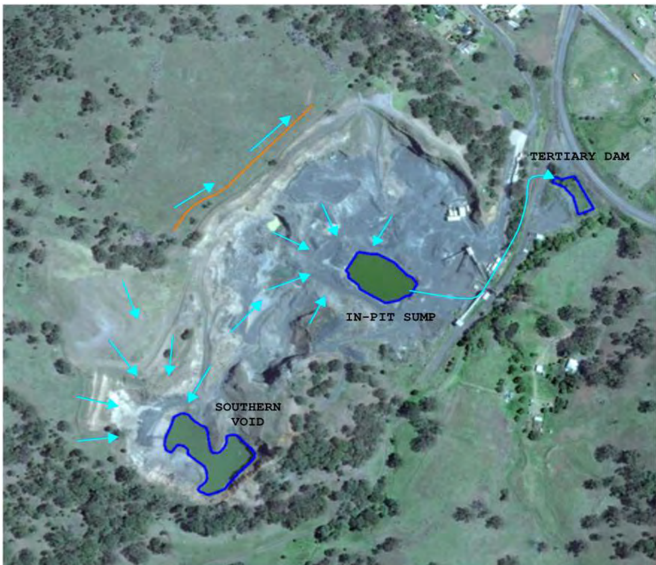
Figure 3: Surface Water Management
