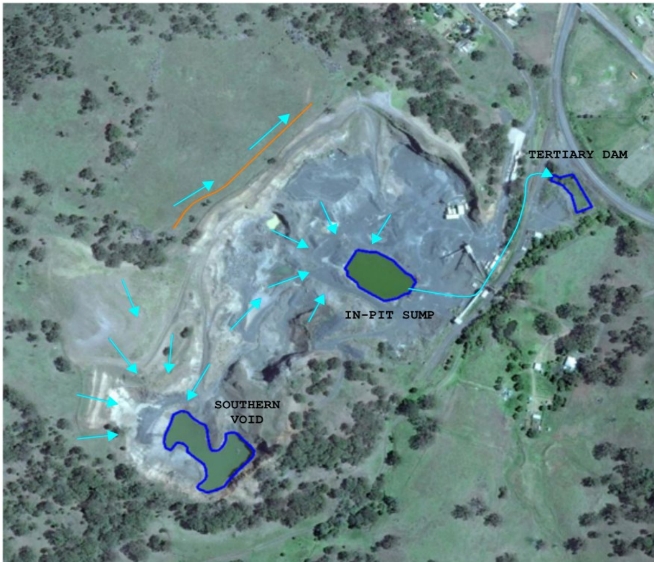
Figure 3: Surface Water Management
